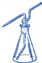
Washing bottle, Conical form, With ground-in glass stopper
