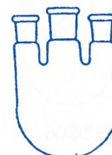
Flask, With four necks, Standard ground mouth
