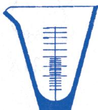
Measuring graduated, conical, with graduation
