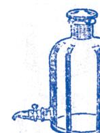
Filtering flask, Clear glass with upper tubulature Boro 3.3 Glass
