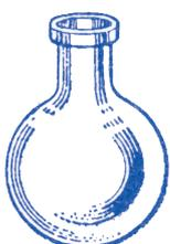
Boiling flask, Round bottom with thick and short neck
