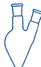
Flask, Pear shape, With two necks, Standard ground mouth
