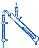
Semicro kjeldahl distilling apparatus
