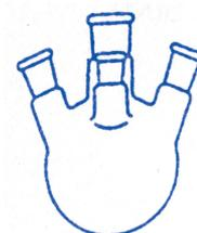
Flask, With four necks, Standard ground mouth
