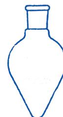
Flask, Pear shape, With two necks, Standard ground mouth
