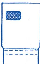
Filter crucible (Gooch crucible), with fritted disc suitable for filter funnel and flask
